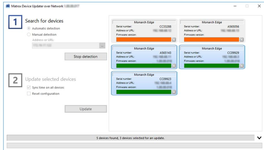
*More info:* Select **Sync time on all devices** to synchronize the internal device clocks across all updated devices. Select **Reset configuration** to reset the encoder settings of the device(s).
