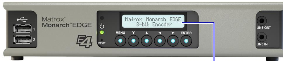
When not being used (idle mode), the Monarch EDGE LCD screen will not display information. Otherwise, it will scroll through the device's status (e.g. IP address, MAC address, etc).
