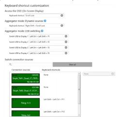
You can assign keystroke combinations in the **Keyboard shortcut customization** screen. This screen appears when you select **Keyboard shortcuts** in the settings screen for a receiver. You can open the settings screen by either right-clicking the receiver tile and selecting **Open settings**, or by doubleclicking the receiver tile.
