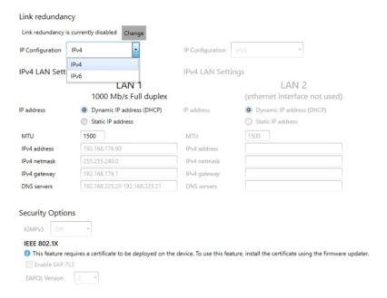
Note: When the IP address or the method of assigning an IP address to a device changes, you need to reboot the device for the changes to take effect.
