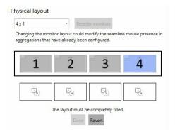
**3** Drag and drop the displays one by one into their correct position on the layout.
