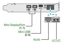
Note: Connect one end of the USB cable included with your product to the mini USB connector on your transmitter card. Connect the other end of your cable to a USB connector on the motherboard of your system. Make sure your connectors are properly connected.
