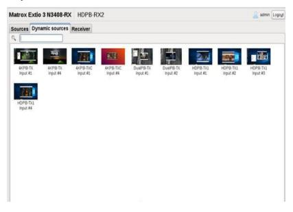
**3** To switch to the transmitter associated with the stream, click **Connect** (or, double-click the target stream). The selected stream is now displayed on the monitor assigned with dynamic sources.
