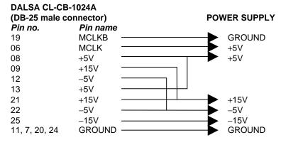
**NOTE:** it is very important that all the GROUNDs of the camera be connected together to the POWER SUPPLY GROUND, and to the GROUND of the Matrox Genesis. Do not use the cable shield as a ground, instead always use the ground pin of the power supply.
