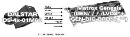
\*Matrox Genesis main board with LVDS grab module Matrox LVDS digital input board
